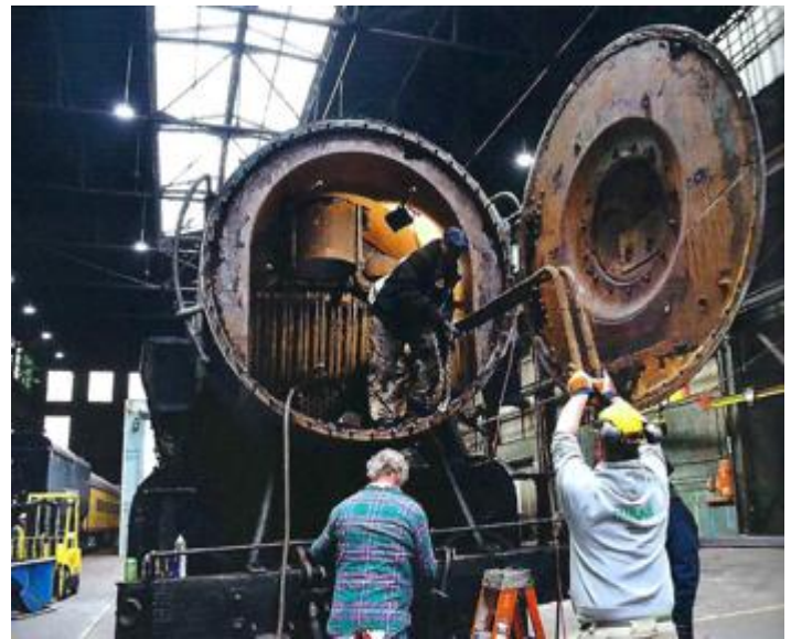
Flues are removed from the Challenger #3985
